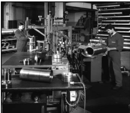
Assembly of piston accumulators
